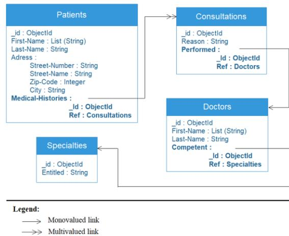
Figure 7: Excerpt from the physical model of data.
