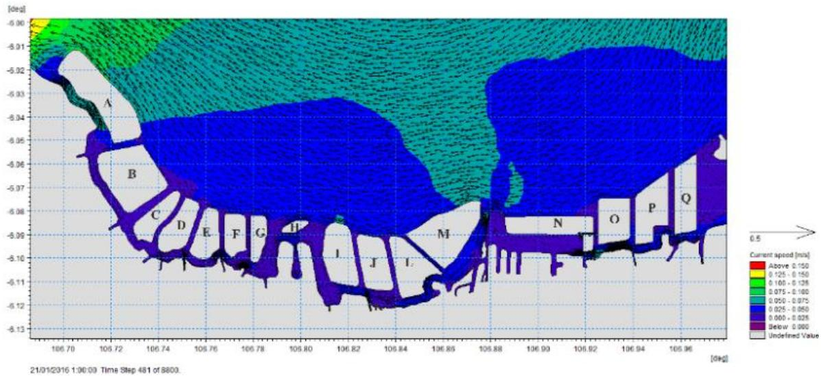
Figure 5. Current pattern at the highest tide in the west season: a) post reclamation b) master plan
