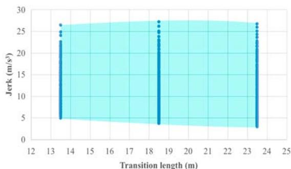
Figure 9: Maximum jerk envelope for different greyhound transition lengths from the second scenario simulations depending on track bend radius and distance of the race start from the bend.
