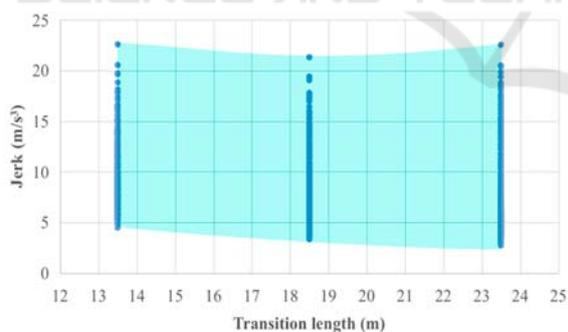
Figure 11: Maximum jerk envelope for different greyhound transition lengths from the third scenario simulations depending on track bend radius and distance of the race start from the bend.
