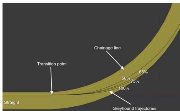
Figure 5: Greyhound transitioning into the bend with no track bend transition where the smallest radius turn is the transition exit radius.
