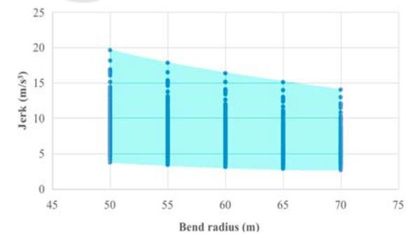
Figure 8: Maximum jerk envelope for different bend radius from the first scenario simulations depending on greyhound transition length and distance of the race start from the bend.
