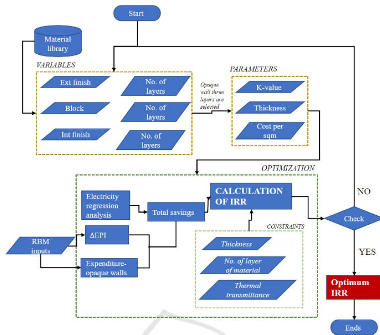
Figure 3: Optimization process flowchart.
