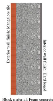
Figure 4: Cross-section image of a wall section using the most recurring material selection after optimization.
