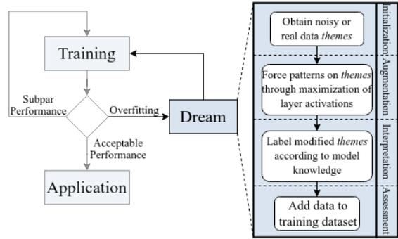
Figure 3: Overview of the neural network’s workflow, with the dream stage being used as a mechanism to tackle overfitting.
