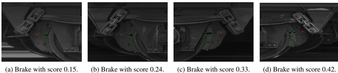
Figure 4: Result of keypoint detection on cargo wagon brake and scored brake pads.
