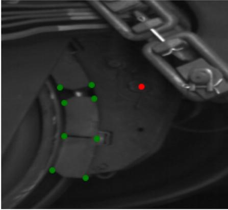
Figure 3: Keypoints of partially occluded brake. Brake pads border keypoints in green. Brake axis keypoint in red.
