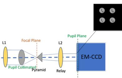
Figure 2: Pyramid WFS scheme.
