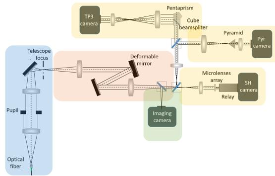
Figure 4: Mounting proposals for each module of the ALIOLI instrument.
