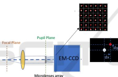
Figure 1: Shack-Hartmann WFS scheme.
