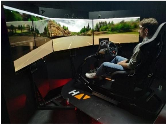
Figure 2: Example of HAV simulating the behaviour of an autonomous vehicle in a highway.
