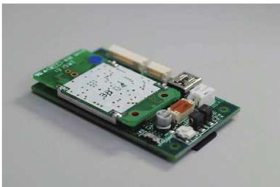
Figure 3: Sensor nodes for real-time vital sensing during exercises.
