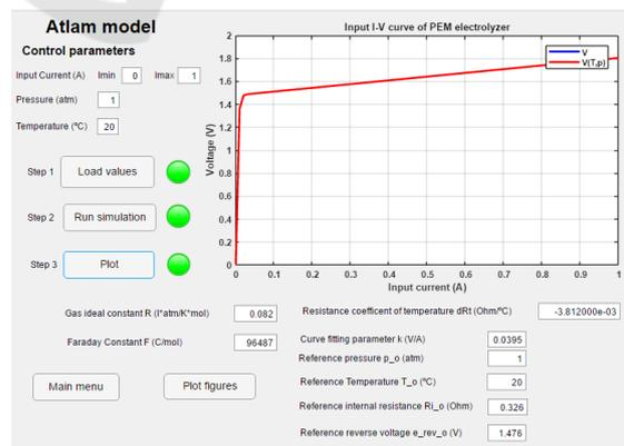
Figure 9: Input I-V curves at 20 °C and 1 atm represented in the GUI.
