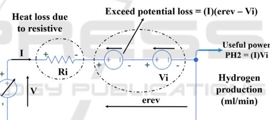
Figure 2: Equivalent circuit model for a single PEMEL.
