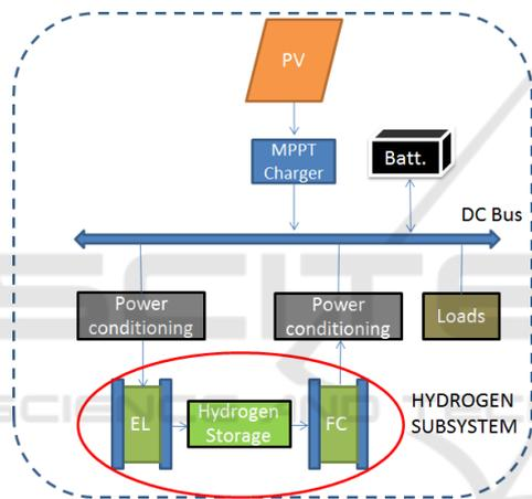
Figure 1: Schematic diagram of the stand-alone microgrid with hydrogen subsystem.
