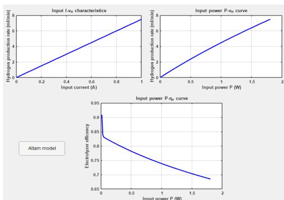
Figure 10: I-vH, P-vH and P-ηe curves simulated in the GUI.
