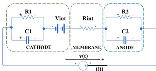
Figure 3: Equivalent circuit scheme of the PEMEL.
