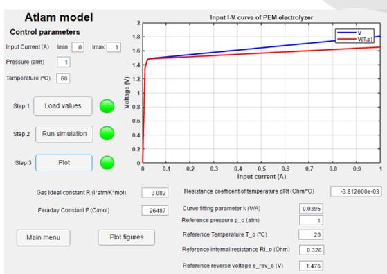
Figure 11: I-V curves at  $60\text{ }^\circ\text{C}$  and 1 atm represented in the GUI.
