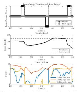
Figure 4: Lane change decisions, Lane utilities and vehicle speed during a part of autonomous driving.
