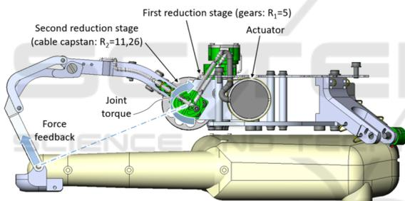
Figure 12: Force feedback generated on fingertips.
