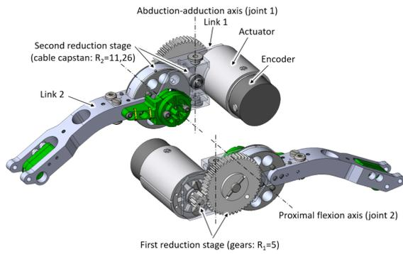
Figure 11: Actuation units.
