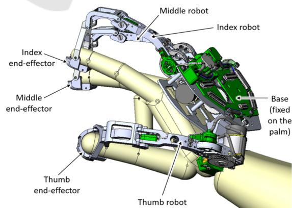
Figure 6: Overview of the tri-digital master glove.
