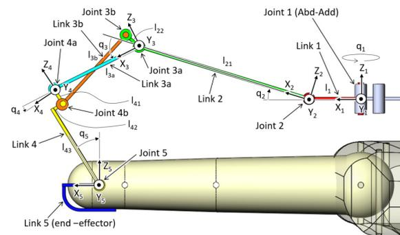
Figure 9: Kinematic model of the robots. A frame  $R_i=(O_i, X_i, Y_i, Z_i)$  is associated with each link, with its origin positioned on the joint axis,  $q_i$  is the rotation around joint  $i$ , and  $l_i$  (resp.  $l_{i1}, l_{i2}$ ) designates the length of link  $i$  (resp. of different parts of link  $i$ ).
