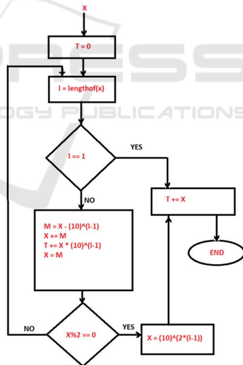
Figure 3: An Efficient Algorithm for N-bit Binary Squaring Approach utilising amalgamation of Vedic Sutras
