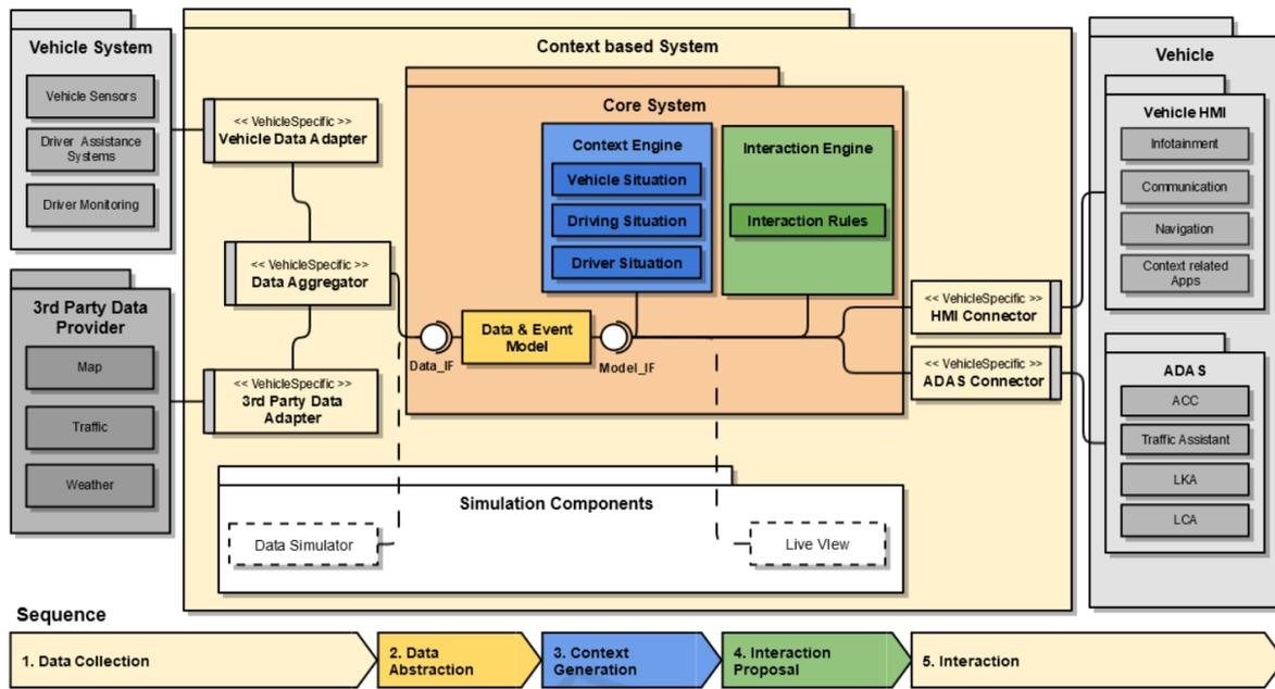
Figure 1: General Architecture. It is comprised of five main steps: 1) Data Collection; 2) Data Abstraction; 3) Context Generation; 4) Interaction Proposal; and 5) Interaction. In each step, a number of components connected to each other perform dedicated tasks.
