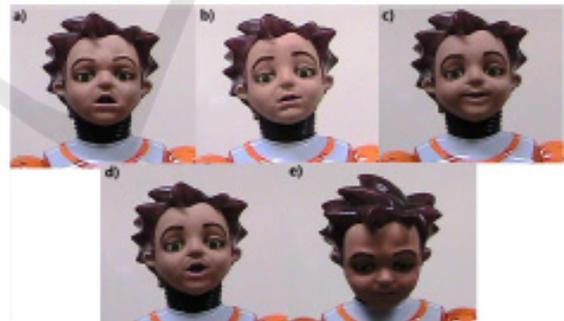
Figure 3: The different facial expressions displayed by the robot ZECA: a) anger, b) fear, c) happiness, d) surprise, and e) sadness (Soares et al., 2019).
