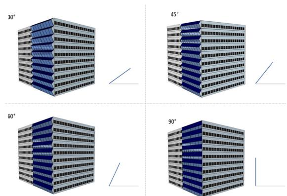
Figure 3: Illustration showing various tilt angles on building façade.
