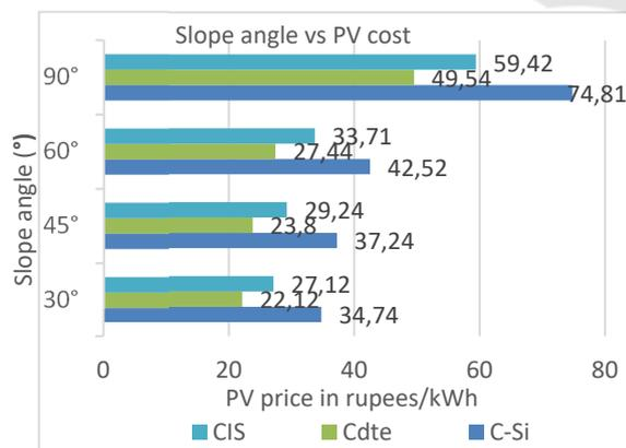
Figure 6: Graph showing a comparison between PV technology, price in INR and the PV tilt angle.
