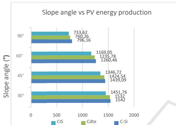
Figure 5: Graph showing a comparison between PV technology, yearly energy production (kWh) and the PV tilt angle.
