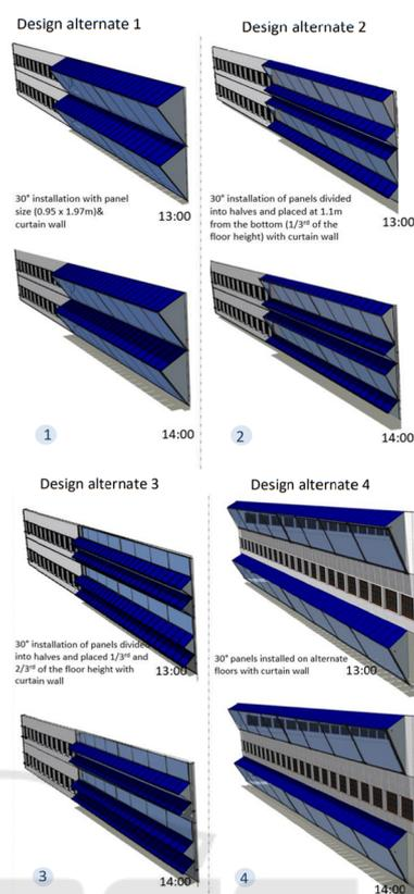
Figure 7: Illustration showing various styles 30-degree PV panels can be integrated on the façade.
