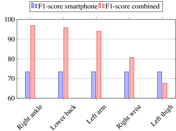
Figure 6: Recognition improvement if the smartphone is combined with each body-worn standalone IMU device.
