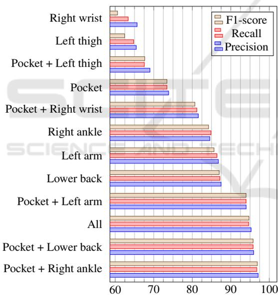
Figure 4: Recognition performance for the different sensor combinations. *Pocket* describes the smartphone in the right pocket.
