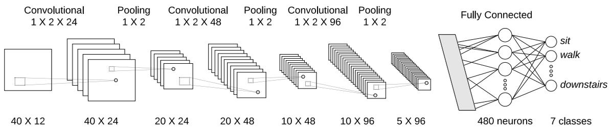
Figure 3: CNN architecture for classification of data from two IMUs.
