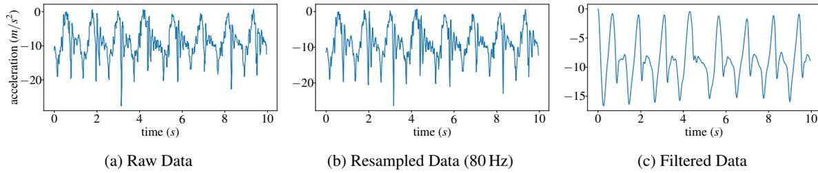
Figure 2: Preprocessing of acceleration data along the x-axis shown on an example upstairs activity recorded at the left thigh.
