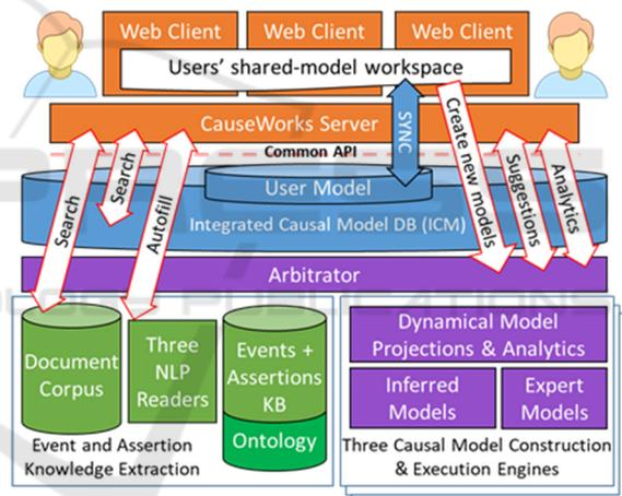
Figure 3: CauseWorks system architecture includes a federation of three NLP readers and three causal modelling framework performers. The ICM combines all models into a single database, and the Arbitrator routes work among readers and frameworks. Analytics, search, and other tools are exposed to CauseWorks as services via a common API.
