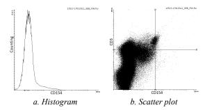
Figure 1: Flow cytometry data examples. (a) a histogram of the number of cells measured at different fluorescent intensity values for the CD154 marker. (b) a scatter plot of the fluorescent intensity values for the CD3 versus the CD154 marker, used for identifying smaller populations, with the quadrant markers demonstrating that most cells have a low response to both CD154 and CD3.
