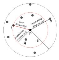
Figure 5: The difference between core-distance and reachability-distance, given  $\epsilon$  and MinPts = 5.
