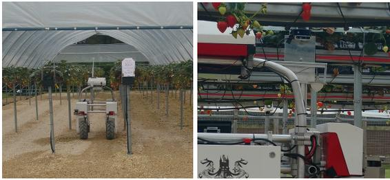
Figure 1: The strawberry farm, with a robot roaming in the tabletop rows collecting data (left). The sensor set-up used for data collection (right).
