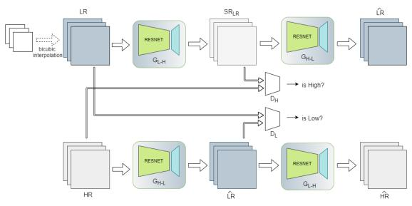
Figure 6: Proposed CycleGAN architecture using 6 residual blocks ResNet;  $G_{L-H}$  and  $G_{H-L}$  represent generators from lower to higher and from higher to lower resolution respectively.  $D_H$  and  $D_L$  represent the discriminator for each resolution.
