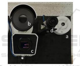
Figure 2: Panel with the cameras: a) Axis Domo P1290 (LR); b) Axis Q2901-E (MR); c) FC-6320 FLIR (HR); d) Basler visible spectrum camera, which is not used in the current work.
