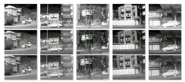
Figure 7: Examples of thermal images used for training. (top) LR images from Axis Domo P1290. (middle) MR images from Axis Q2901-E. (bottom) HR images from FC-6320 FLIR.
