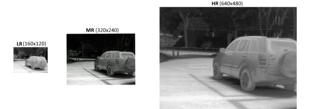
Figure 1: Example of thermal images acquired by each camera. (left) LR image with 160x120 native resolution from Axis Domo P1290. (middle) MR image with 320x240 native resolution from Axis Q2901-E. (right) HR image with 640x480 resolution from FC-6320 FLIR (native resolution 640x512).
