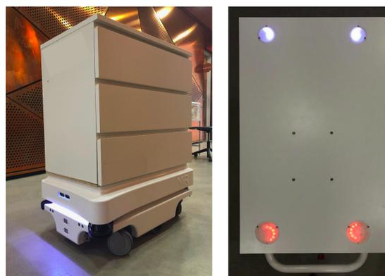
Figure 1: Robot test platform used for the experiments (left); top view of the robot with standard car light pattern (right).
