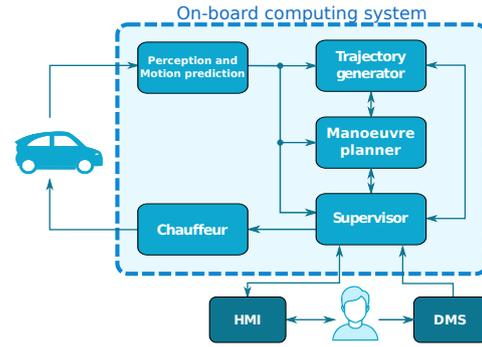
Figure 1: Autonomous driving architecture for Autopia Program.
