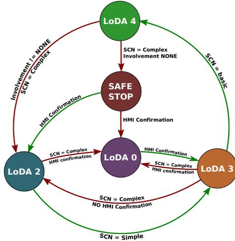
Figure 5: FSM for automation level.
