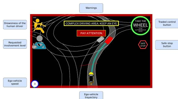
Figure 9: HMI warning due to low attention from the human operator.
