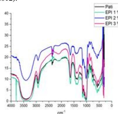
Figure 2: FTIR spectrum of cross-linked starch with various concentration of epichlorohydrin (1%, 2%, 3%).
