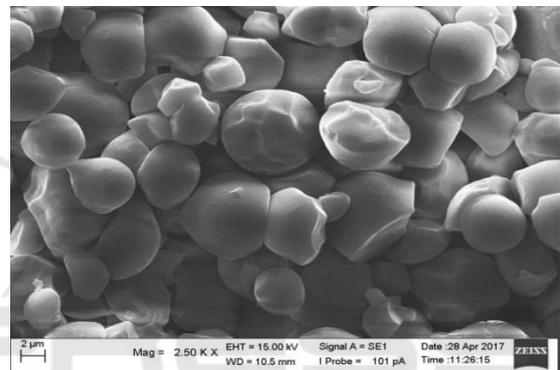
Figure 4: The surface morphology of cross-linked starch with magnification 2000x.
