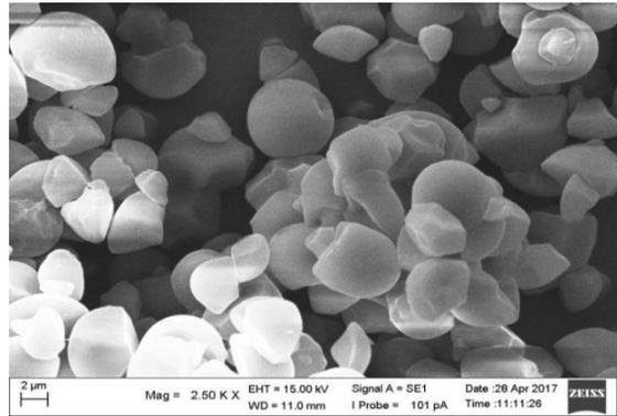
Figure 3: The surface morphology of breadfruit starch with magnification 2000x.
