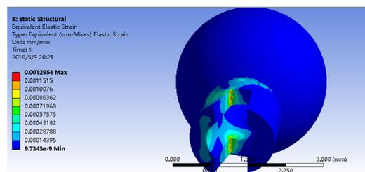
Figure 11. Improved nozzle stress cloud diagram.
