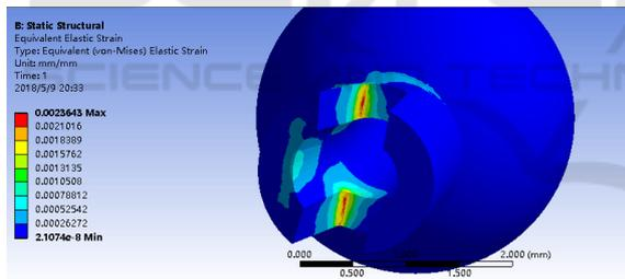
Figure 8. Nozzle deformation before improvement.
