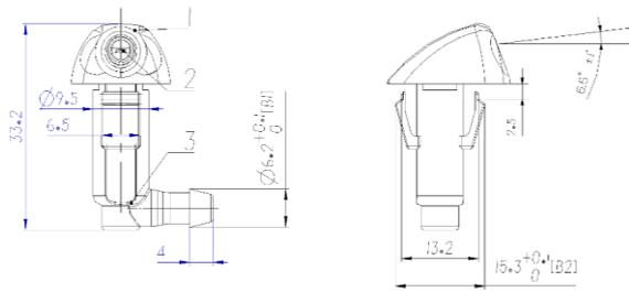
Figure 4. Nozzle Angle change diagram.
