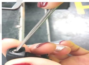
Figure 1. Nozzle regulating method.
