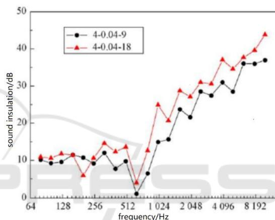
Figure 3. Comparison of sound insulation of honeycomb panels with different heights.
