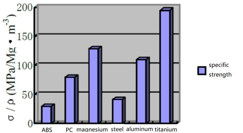
Fig 2. Comparison of specific strength between magnesium alloy and other metal materials.
