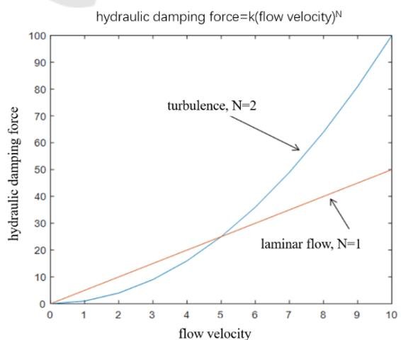
Figure 1. Relation of flow speed and damping force.
