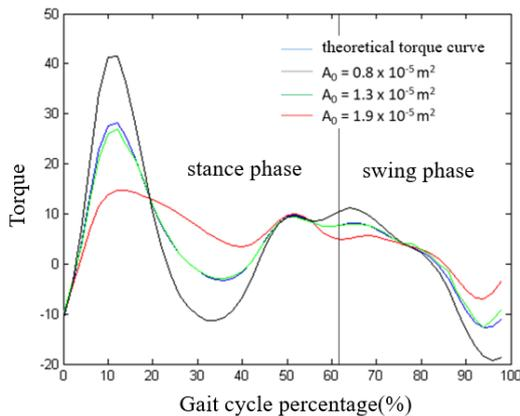
Figure 6. Knee theoretical torque and damping torque in different flow area.
