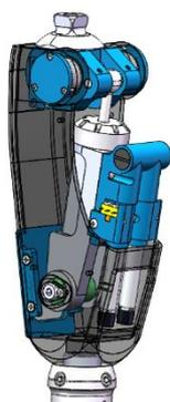
Figure 2. Knee prosthesis structure.
