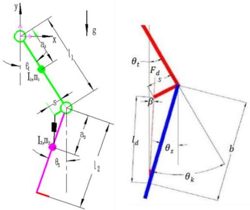
Figure 3. Dynamics model of lower limb prosthesis.
