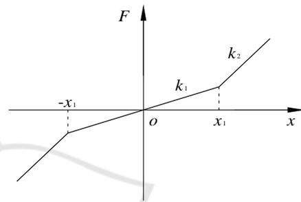
Figure 2. Force characteristic of two stage stiffness spring.
