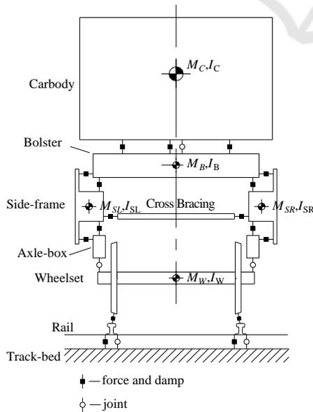
Figure 1. Physical model of railroad car system: side view.
