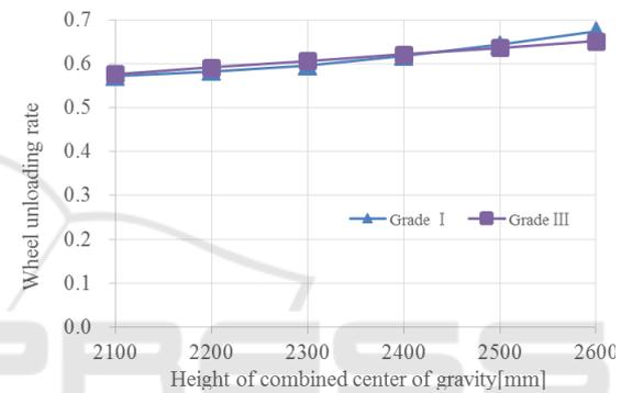
Figure 7. Wheel unloading rate trend.
