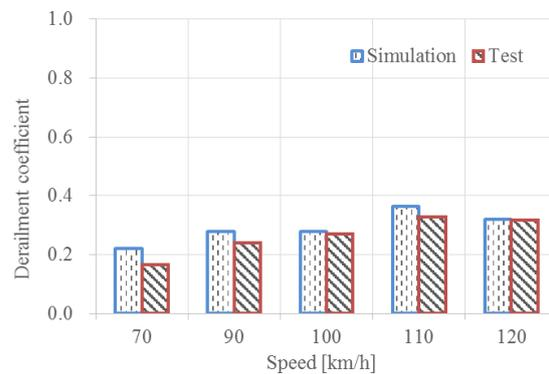
Figure 4. Derailment coefficient compare on tangent track.
