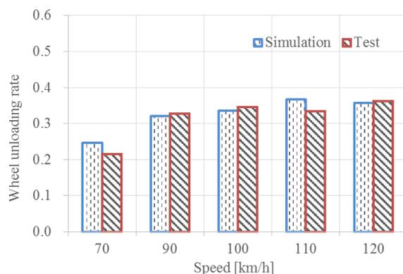
Figure 5. Wheel unloading rate compare on tangent track.
