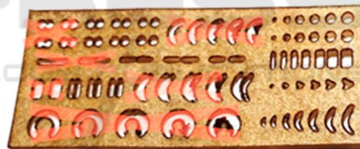
Figure 5. Laser Cut Result (Rawhide)
