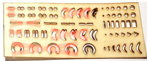
Figure 6. Laser Cut Result (Split Leather)
