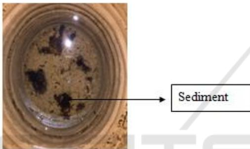
Figure 3: Sediment on Ceramic Membrane.
