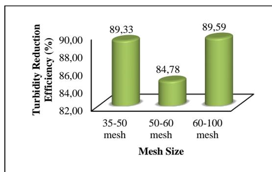
Figure 12: Average Efficiency of Turbidity Reduction on Ceramic Membrane Based on Mesh Size.
