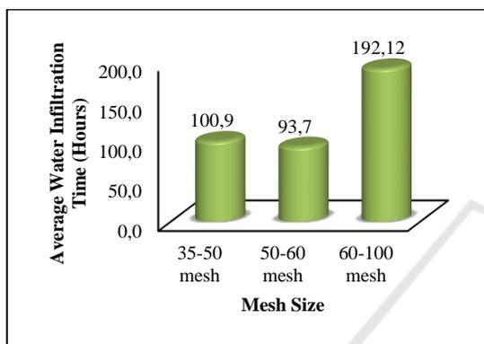
Figure 6: Average Water Infiltration Time on Ceramic Membrane Based on Mesh size.
