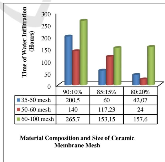
Figure 5: Average Time of Water Infiltration on Ceramic Membrane.
