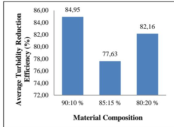
Figure 10: Average Efficiency of Turbidity Reduction on Ceramic Membrane Based on Material Composition.
