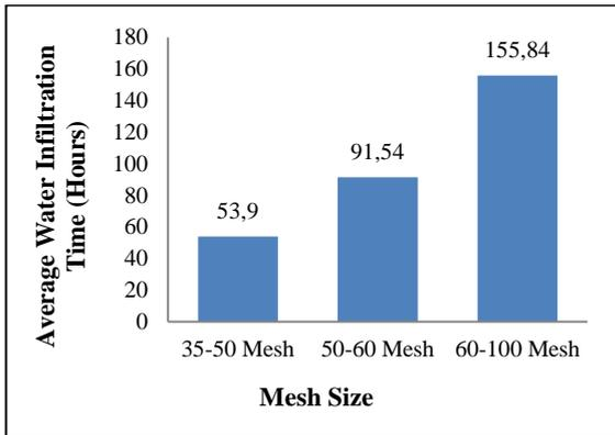
Figure 2: Average Time of Water Infiltration (Hours) Based on Material Size (Mesh).
