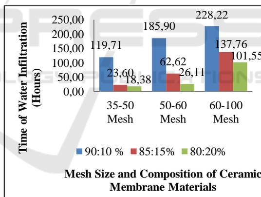
Figure 1: Average Water Infiltration Time (Hours) on Ceramic Membrane.
