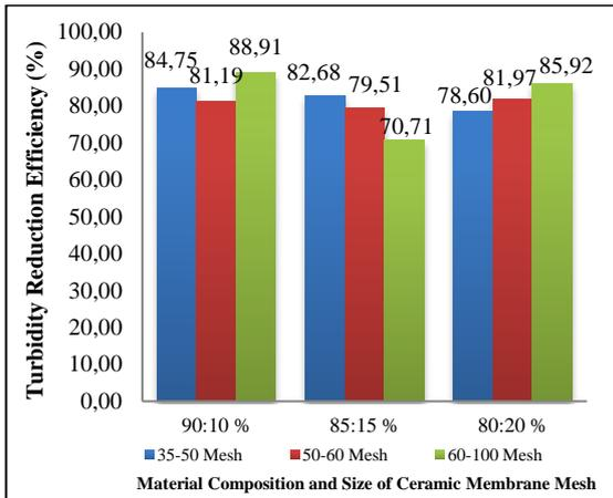
Figure 8: Average Efficiency of Turbidity Reduction in Ceramic Membrane.
