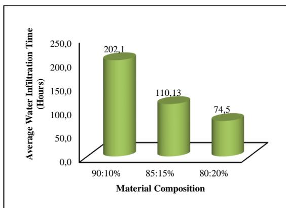
Figure 7: Average Time of Water Infiltration on Ceramic Membrane Based on Material Composition.
