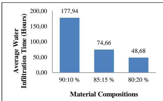
Figure 4: Average Time of Water Infiltration (Hours) Based on Material Composition.
