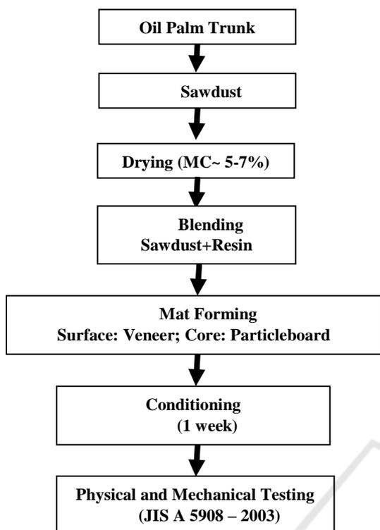
Figure 1: Diagram of com-ply manufacturing.
