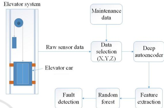
Figure 1: Fault detection approach.
