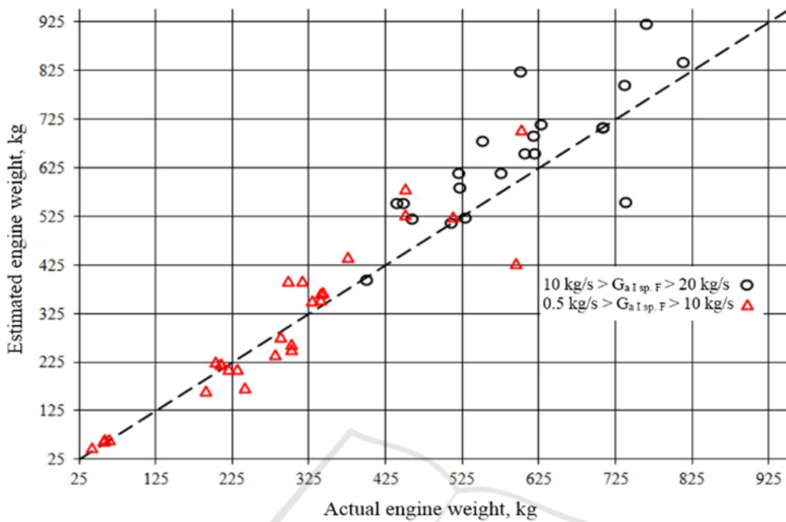
Figure 2: Deviation of actual and calculated values of engine weight for the original model.
