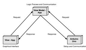
Figure 5: App graphical interface - This diagram shows the MVVM Model implemented in the development of software of the domotic system for people with disabilities. In the model layer the coding of the Arduino was implemented, in the view layer the code of the graphical interface of the APP was implemented and in the model layer the code necessary for the Wi-Fi connection processes of the system was implemented.
