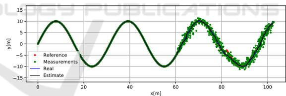
Figure 5: The x,y view of the simulation using the sine trajectory. Midway through the trajectory noise is applied to the position measurements, and then a change lane occurs just before the last corner.
