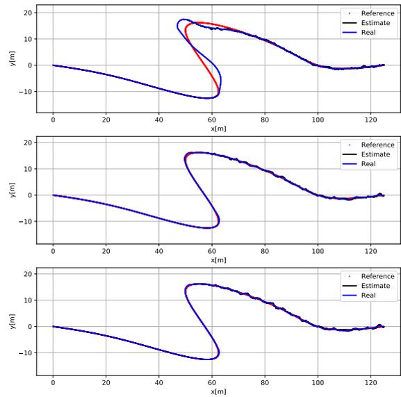
Figure 4: The x,y view of the simulation using the spline1 trajectory and a constant gain model. Midway through the trajectory noise is applied to the position measurements. Above: The first plot with a low gain of 0.1. Middle: The second plot with a high gain of 3.0. Below: The third plot with a very high gain of 7.0.
