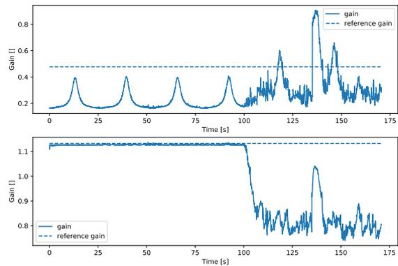
Figure 8: The gain outputted by the neural network in the solid line, and the optimal constant gain value in the dashed line. Above: when trained without using the EKF covariance matrix as input. Below: when trained without using the curvature of the trajectory as input.
