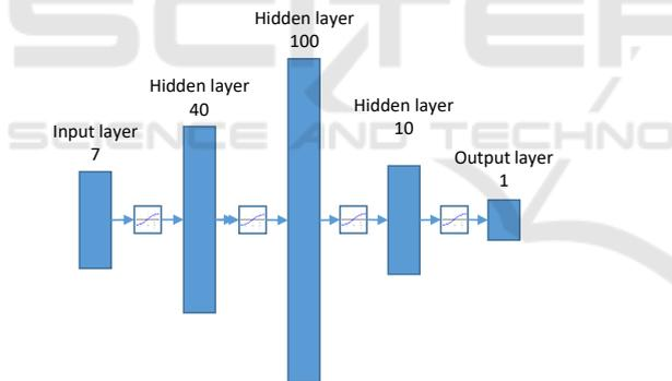
Figure 3: Graphical representation of the used neural network. With 7 neurons in the input layer, 3 hidden layers of 40, 100, and 10 neurons respectively, and 1 neuron for the output layer. all the layers except the output layer go through a hyperbolic tangent function as the activation function.
