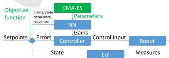
Figure 1: Control bloc diagram of the proposed method. In green is the CMA-ES training method and in blue the control loop with the neural network (NN).
