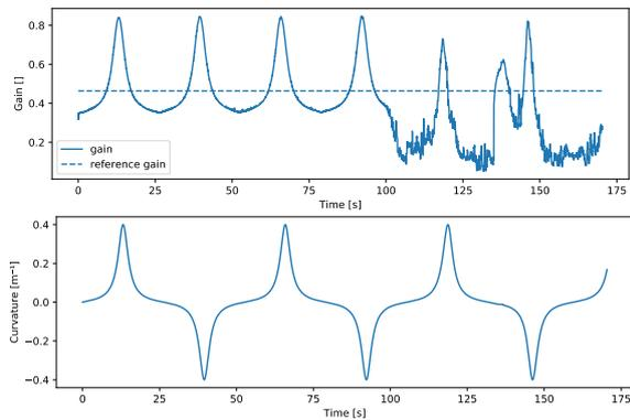
Figure 6: Above: the gain outputted by the neural network in the solid line, and the chosen constant gain value in the dashed line. Below: the curvature of the trajectory over time.
