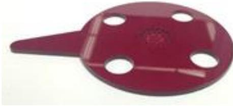
Figure 20: Manufactured flow conditioner.
