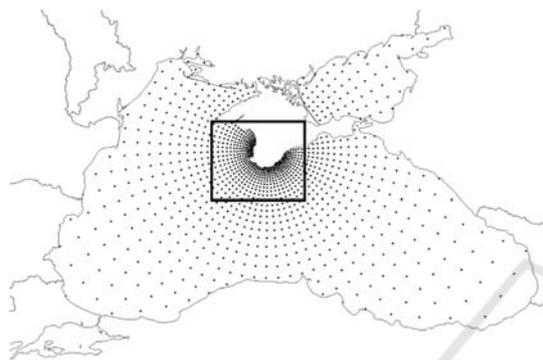
Figure 1: Grid domain of the  $\sigma$ -model of marine circulation INMOM with nonuniform grid near the Crimean Peninsula.
