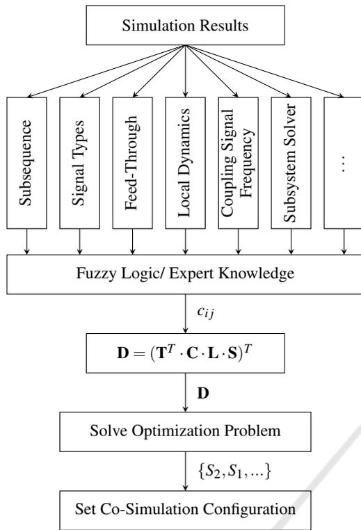
Figure 4: Schematic procedure to get the trigger sequence.
