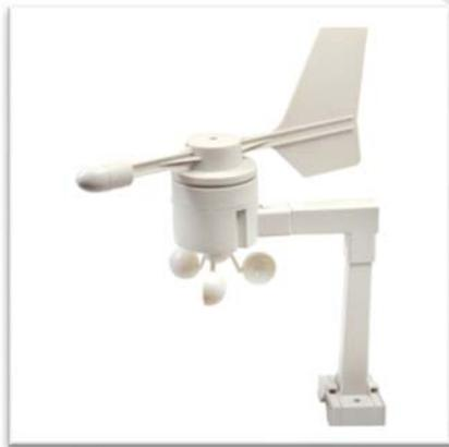
Figure 5: The wind sensor.
