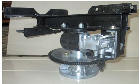
Figure 2: The orientation system, drive motor and chassis.
