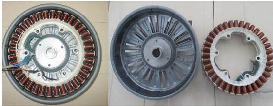
Figure 3: The power generator – left: assembly, centre: rotor and right: stator.
