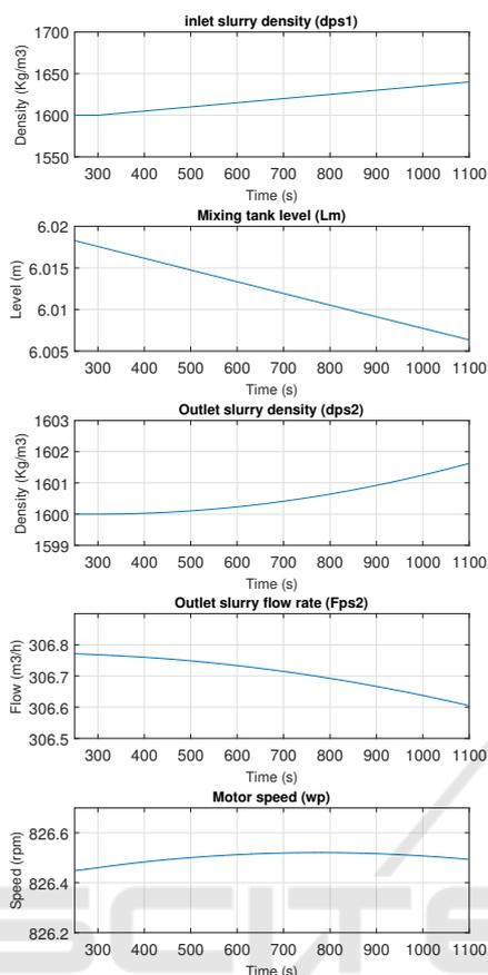
Figure 13: The effect of inlet slurry density small variation. affects the induction motor speed, then a change of the induction motor speed changes the outlet flow rate. That highlights the importance of these parameters in the control strategy design.
