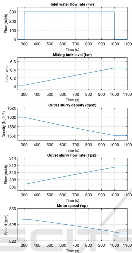
Figure 11: The effect of water flow rate large variation.
