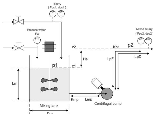
Figure 1: Pump hydraulic application parameters.
