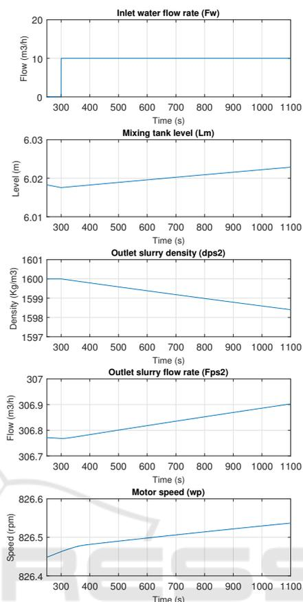
Figure 14: The effect of water flow rate small variation.
