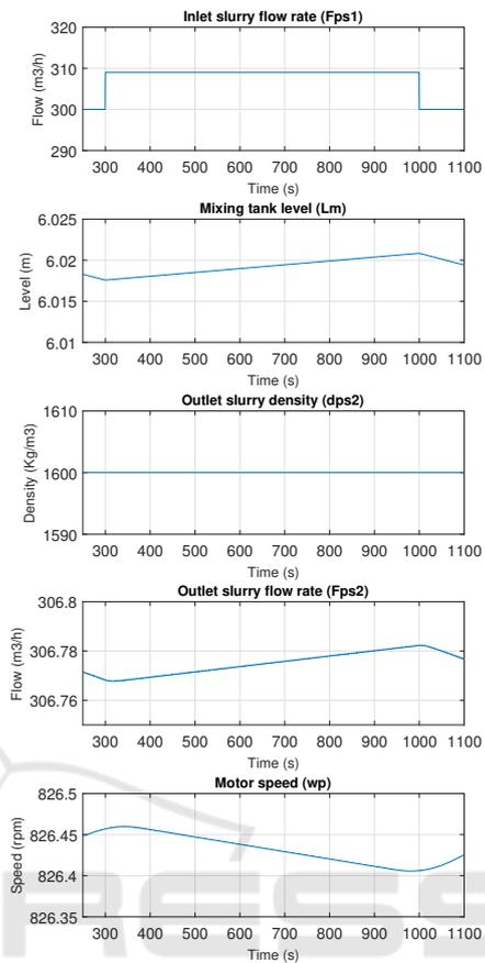
Figure 12: The effect of inlet slurry flow rate small variation.
