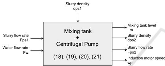
Figure 2: The mixing unit bloc diagram.
