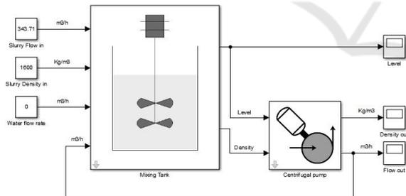
Figure 5: The mixing and pumping unit simulation using Matlab/Simulink.
