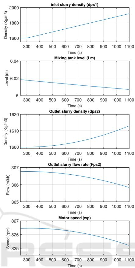
Figure 10: The effect of inlet slurry density large variation. and Nixon, 2010), this increase in the outlet slurry density increases the pump load torque. The rise in load torque decreases the motor speed then the outlet slurry flow rate decreases. Thus, a change in slurry density impacts inversely the outlet slurry flow rate.
