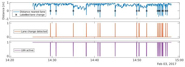
Figure 5: Sequence of a trip on a motorway with two to three lanes for demonstrating the proof-of-concept of the proposed VDMS for scenario identification and system evaluation. *Top:* Distance to nearest line and the manually labelled lane changes. *Middle:* The detected lane changes of the algorithm. *Bottom:* The signal of the onboard Lane Keep Assist System.
