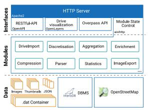
Figure 3: The architecture of the proposed VDMS for managing large-scale test campaigns consists of three layers: *Data, Modules* and *Interfaces*.
