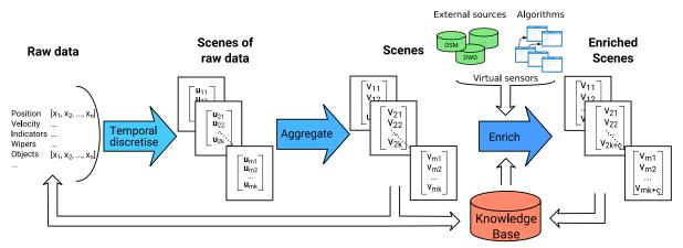
Figure 1: Three stage process for transforming the vehicle sensor data to a series of scenes enriched with additional information from algorithms and external data sources as the foundation for scene-based scenario identification.
