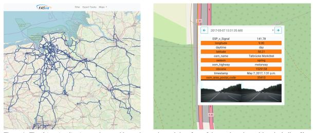
Figure 4: The *drive visualisation* service provides an interactive web-interface of the conducted test drives including filter capabilities for efficient sequence identification and track selection for scene analysis. *Left:* A map of all conducted test drives. *Right:* The same zoomed-in map showing information of a selected scene.
