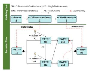
Figure 4: Pattern SEQ-INSTANCES-COP for a collaborative task T.
