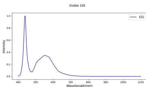
Figure 3: Spectrum of White LED at maximum intensity (100%) obtained with the AvaSoft 2048.
