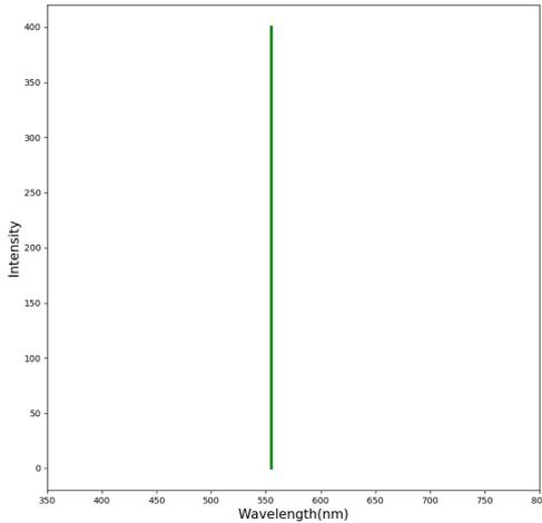
Figure 2: Spectral distribution of an ideal single wavelength light source.
