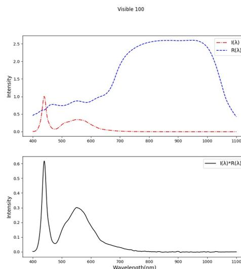
Figure 4: Top - In red is presented  $I(\lambda)$ , the normalized spectral intensity of the light source and in blue is presented  $R(\lambda)$  the relative sensitivity of the photodiode. Bottom - Is presented in black the result of the multiplication of the two curves presented in the Top image -  $R(\lambda) \times I(\lambda)$ , hereinafter referred as Weighted Spectrum.
