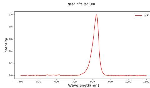
Figure 6: Spectrum of the NIR LED at maximum intensity, (100%) obtained with the AvaSoft 2048.
