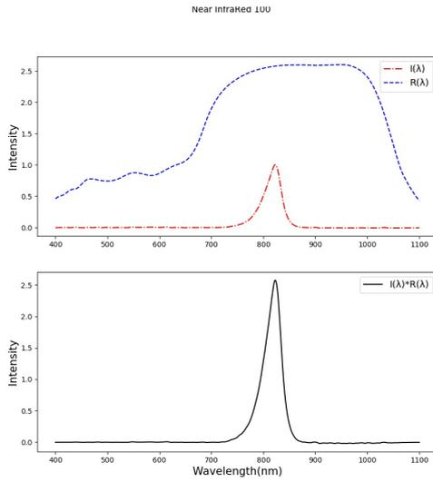
Figure 7: Top - In red is presented  $I(\lambda)$ , the spectrum of the light source and in blue is presented  $R(\lambda)$  the relative sensitivity of the photodiode. Bottom - Is presented in black the result of the multiplication of the two curves presented in the top image -  $R(\lambda) \times I(\lambda)$  - Weighted Spectrum.
