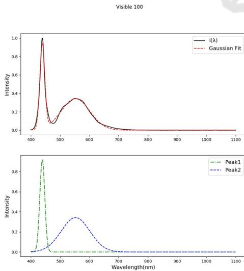
Figure 5: Top - In black is presented  $I(\lambda)$ , the spectrum of the light source and in red is presented the Gaussian Fit function. Bottom - Peaks are individually presented, the first in green and the second in blue.
