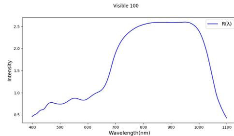
Figure 1: Spectral Response of the PD300-3W with the replaceable filter in.  $R(\lambda)$  is the relative sensitivity of the photodiode for the wavelength  $\lambda$ .
