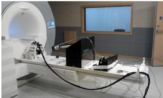
Figure 1: MR-compatible driving system.
