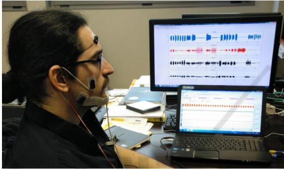
Figure 2: Recording set-up for Signal acquisition of speech, accelerometry and surface electromyography (sEMG).
