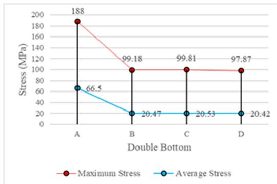
Figure 8: Graph of maximum stress comparison and average stress on double bottom variations.
