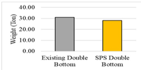
Figure 9. Graph of comparison of estimated weight of double bottom construction.
