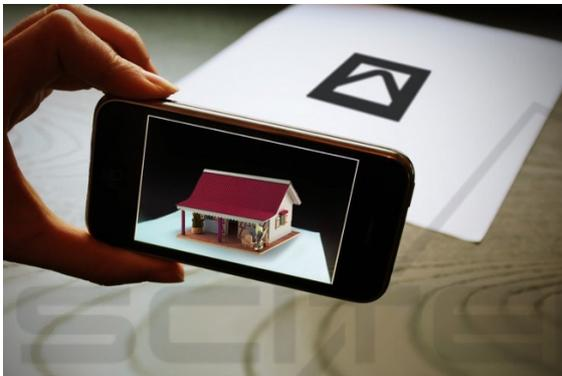
Figure 1: example of marker-based AR
