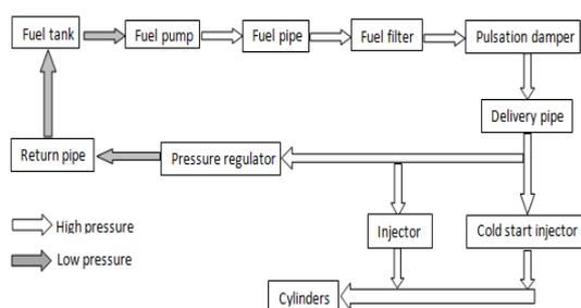
Figure 5: Fuel delivery scheme in electronic fuel pump system.
