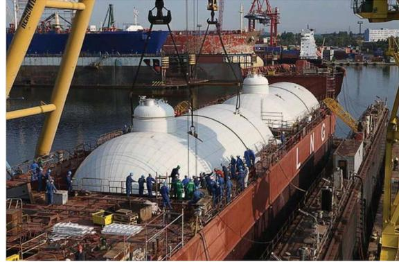
Figure 2: A Type C tank being installed.
