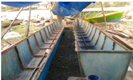
Figure 7: Frame installation result.
