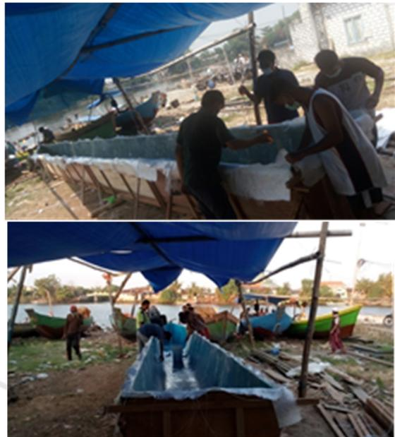
Figure 6: FRP Lamination Process.
