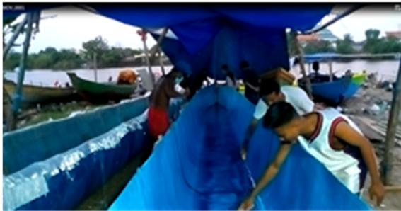
Figure 5: Gel Coating Process.
